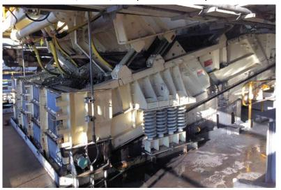
New GK 3.6m x 6.1m 800t/hr two mass cascade deck D&R coal screen being commissioned in a major Qld Bowen Basin coal mine, July 2016. The screen consistently performs better than allowed spec of 0.4kg/t magnetite in discharge, from densities of 1.4 up at full flow.
